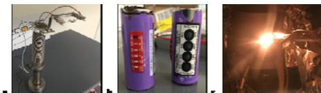
Fig. 2 a. In-house engineered and assembled prototype BPD unit shown before experiment, b. Type 26650 LiPO4 batteries used as the power source shown after experiment, c. The energized BPD filament during the demonstration experiment under high-vacuum.
