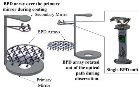
Fig. 1. Artist rendition of a method for coating a Cassegrain-style telescope concept using the battery-powered deposition (BPD) units fixed in a hexagonal array and a single BPD unit up close.
