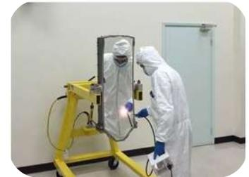
Fig. 4. Inspection of silver coating at ZeCoat Corporation
